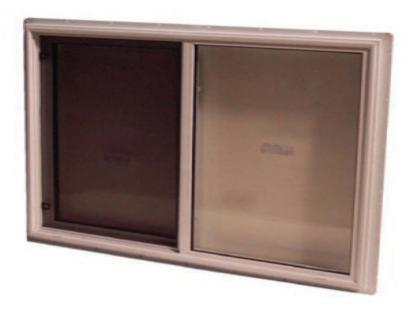
TerraStar Building Products offers two in stock sizes of the thermal pane sliders 46"x 36" and a 46"x 24" (custom sizes available through special order). Each window is built with a J-trim frame that allows the G-Rib profile to be installed with no cut edges visible. It is advised to use a drip trim on the top of the window to prevent any water infiltration.
